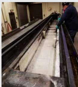
UL tunnel pre burn
