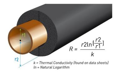
Based on this equation, the R-Value gets larger as the insulation thickness increases **but also** as the pipe sizes gets smaller.
