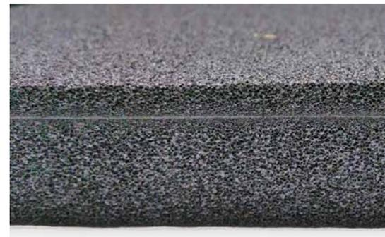
*CGR laminated multiple plies of thin foam together to meet the OEM's custom thickness. multiple plies of thin foam together to meet the OEM's custom thickness.*
